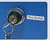
This safety feature enables operators to keep the laser locked to avoid unanthorized
